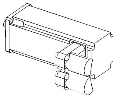
*Can be mounted straight or offset by  $45^\circ$ .
