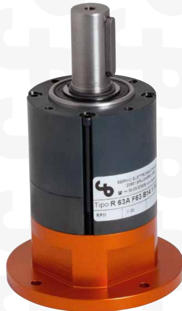
Epicicloidal reduction gearbox with a sintered steel frame, anodized aluminium flange, output shaft supported by two ball bearings Permanent greasing
