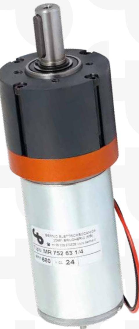
Length "L" of the gearmotor as a function of reduction and output number of revolution with the standard motor 752 40 output W 2900 Rpm loadless, 12 or 24 Vdc. Starting current 7 A (14A x 12 Vdc).
