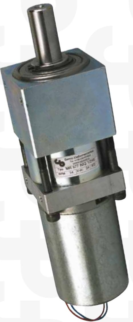
*The standard motor 977 130 output W 2900 Rpm loadness, 24 Vdc. Starting current 38 A.*
