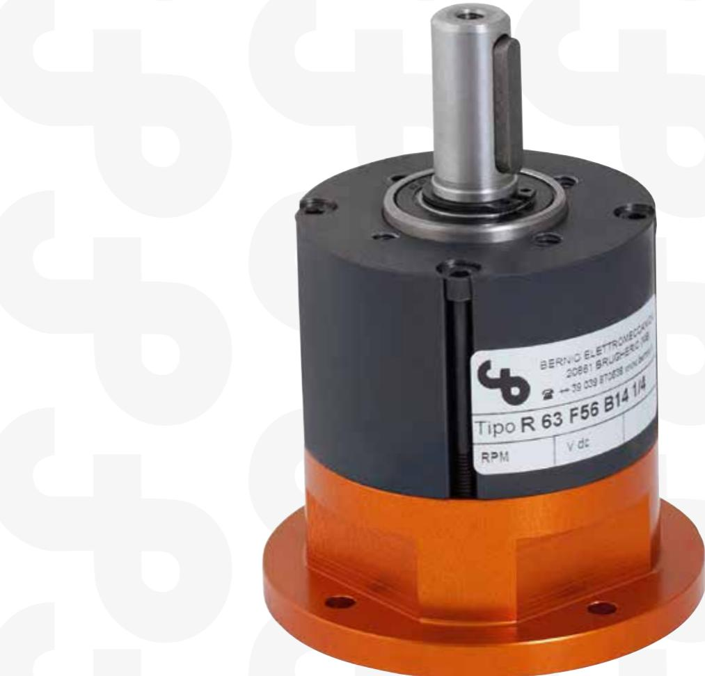
Epicyclic reduction gearbox with a sintered steel frame and, anodized aluminium flange derlin and sintered steel gears, output shaft supported by two ball bearings. Permanent greasing Max forces, which may act on the output shaft: Axial 300 N Radial 400 N on the end of output shaft Max speed advised at the reduction gear 4000 R.P.M. Life in standard condition 4000 hours. Right to be connected with IEC F 56 B 14 motor.
