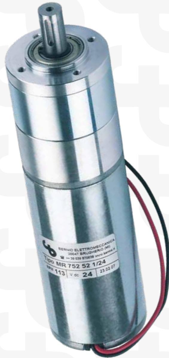
Length "L" of the gearmotor as a function of reduction and output number of revolution with the standard motor 752 40 output W 2900 Rpm loadness, 12 or 24 Vdc. Starting current 7 A (14A x 12 Vdc).
