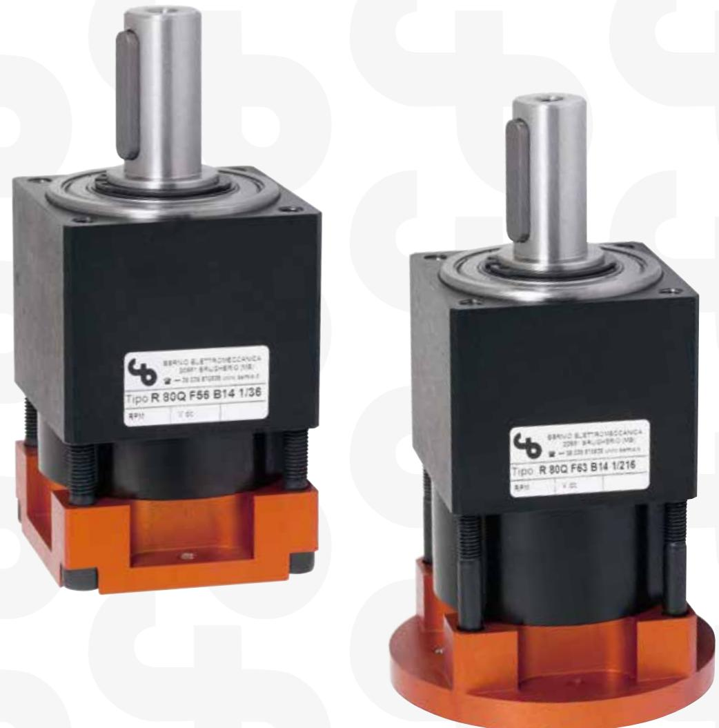
Epicicloidal reduction gearbox zinck plated with anodized aluminium flanges, output shaft supported by two ball bearings Permanent greasing
