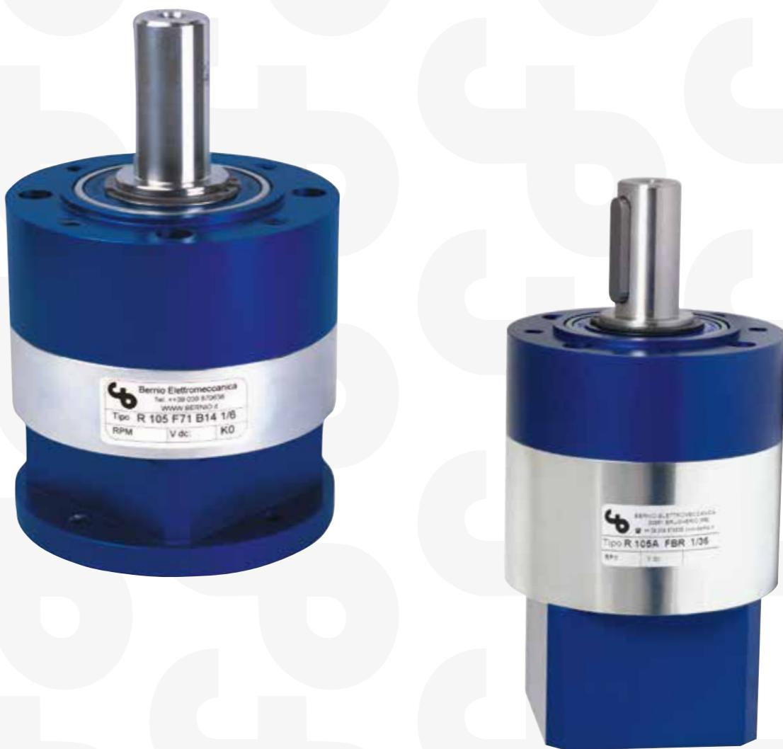
Epicicloidal reduction gearbox zinck plated, with anodized aluminium flanges, output shaft supported by two ball bearings. Permanent greasing
