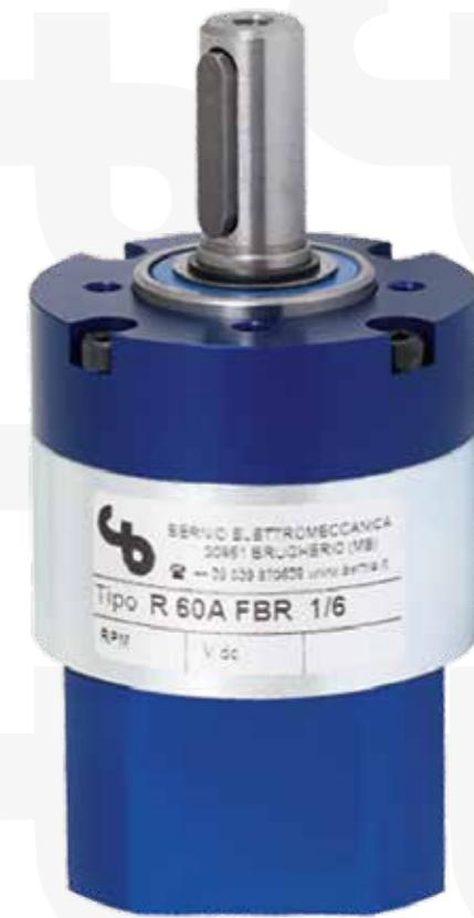
Epicicloidal reduction gearbox zinc plated, with anodized aluminium flanges, output shaft supported by two ball bearings. Permanent greasing.
