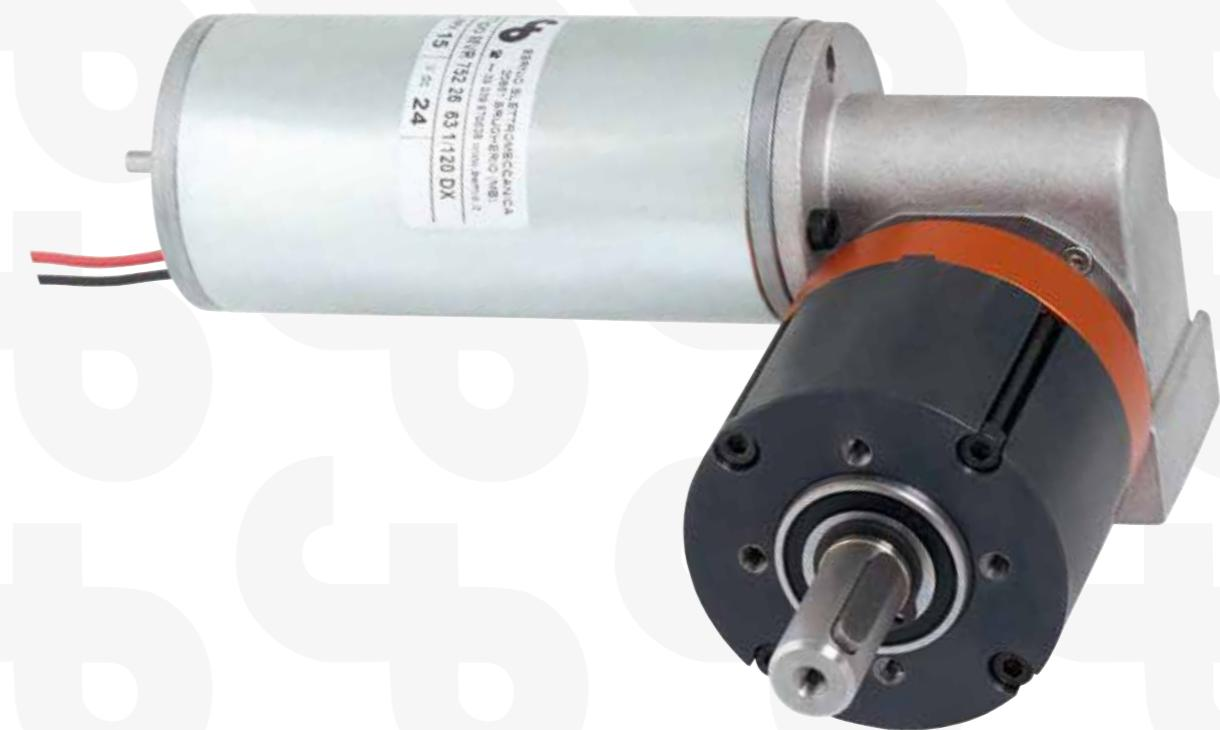
Gear motor with worm screw and standard motor Ø 52 12 or 24 Vdc 2000 RPM output 40 W, with noise suppressor. Starting current 6 A (11A x 12 Vdc)
