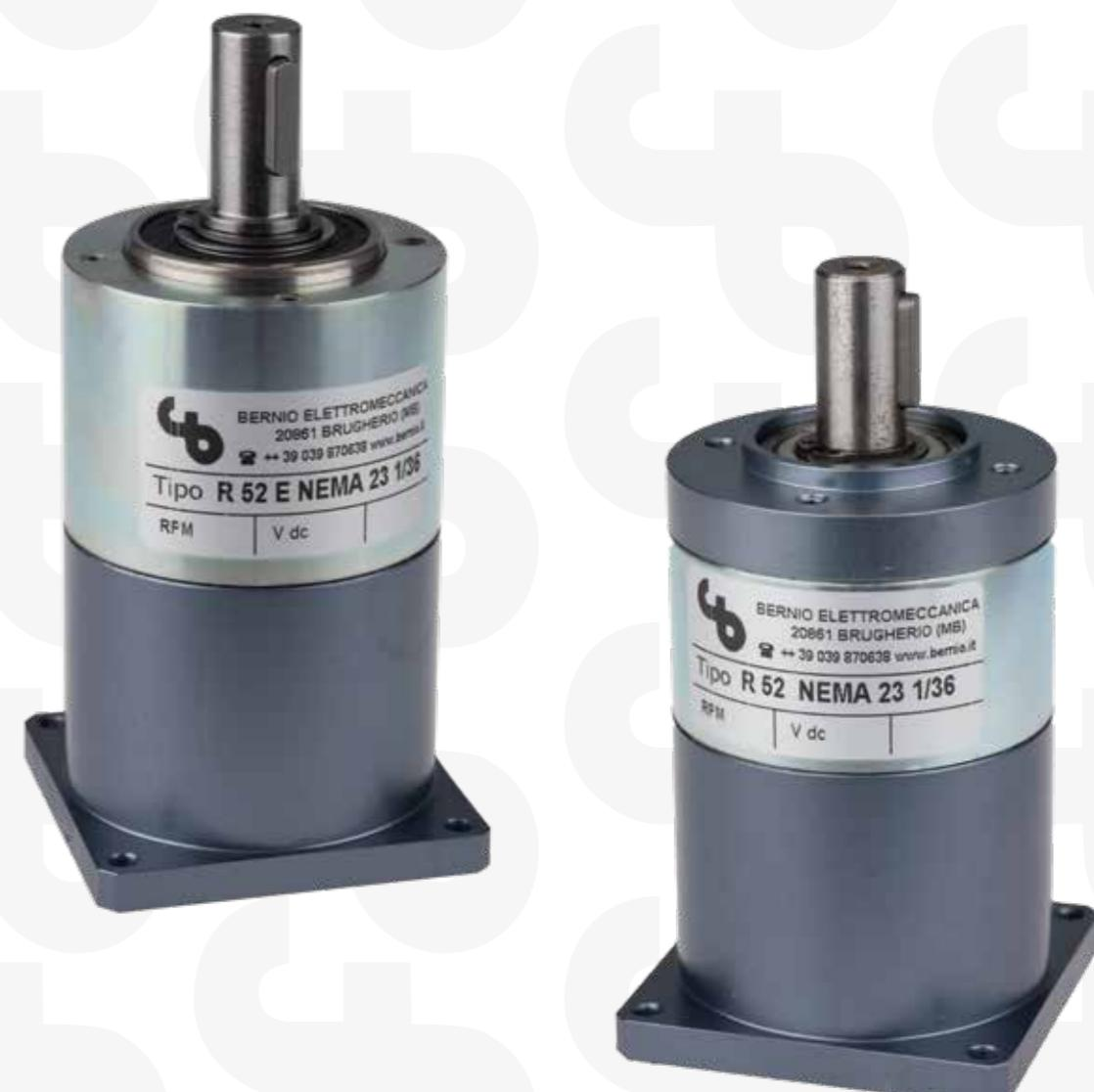
Epicicloidal reduction gearbox with a galvanized steel frame and delrin, sintered steel and hardned steel gear; output shaft supported by two ball bearings max speed at the reduction gear 5000 R.P.M. advised speed 3000 R.P.M.
