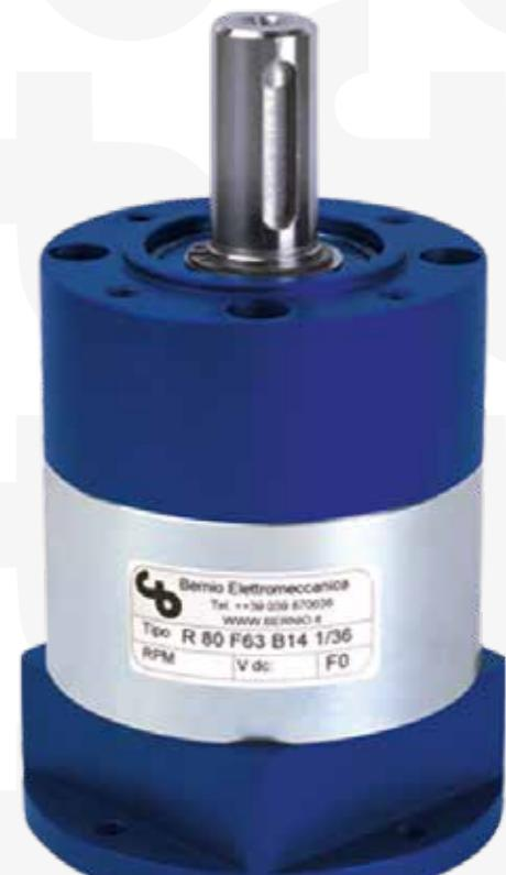
Epicicloidal reduction gearbox zinck plated, with anodized aluminium flanges, output shaft supported by two ball bearings. Permanent greasing.
