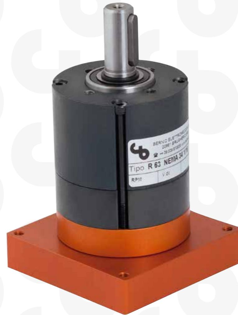
*Epicloidal reduction gearbox with a sterilized steel frame; output shaft supported by two ball bearings max speed at the reduction gear 4000 R.P.M. advised speed 3000 R.P.M.*
