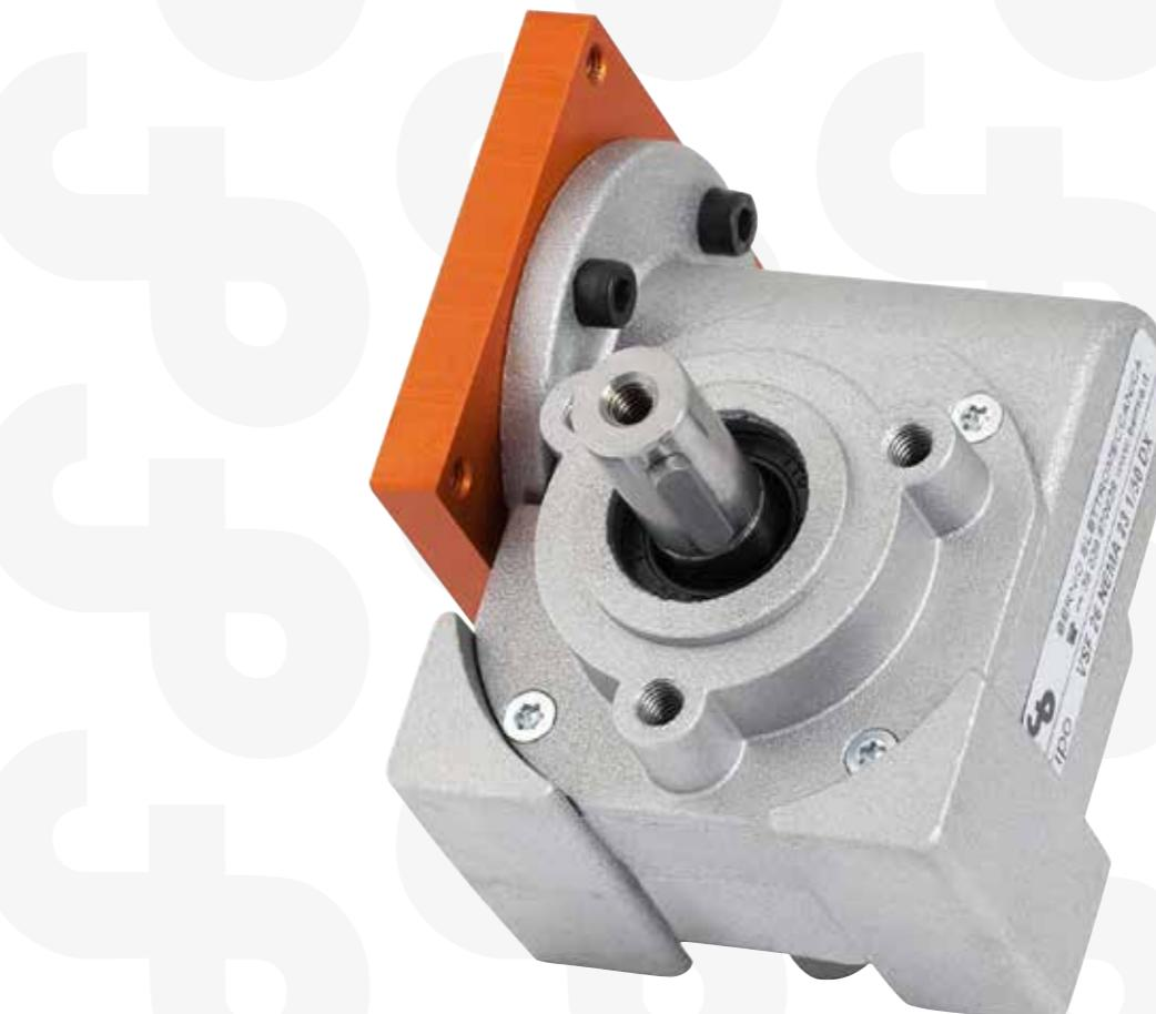
Warm gearbox with a casted aluminium frame delrin, and bakelized cloth gear output shaft supported by two ball bearings
