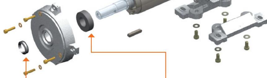
**V-ring or sealing ring for dust protection**
